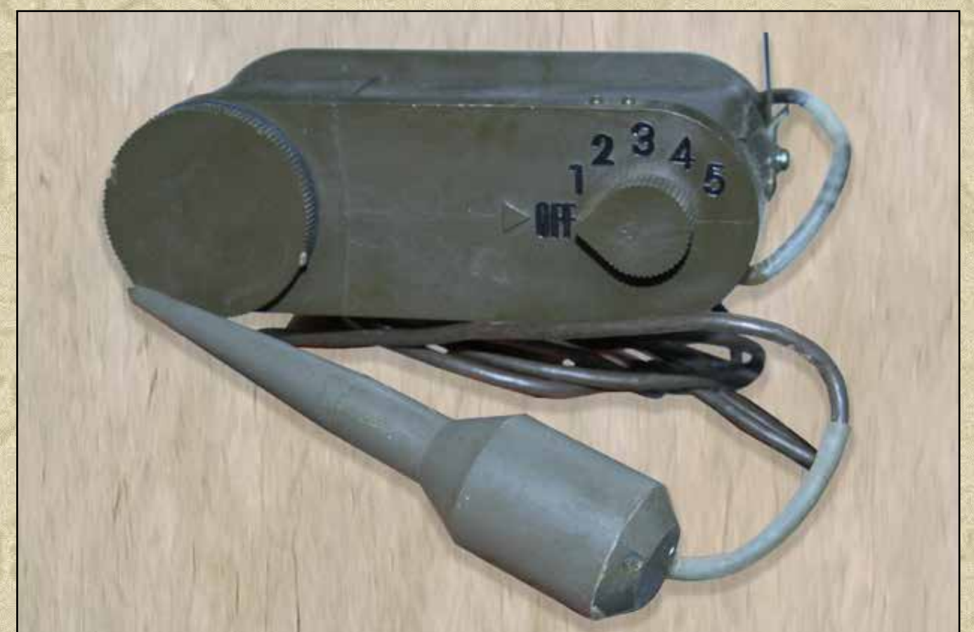
The Patrol Seismic Intrusion Detector uses a spike (seismic sensor) inserted into the ground by hand to guard a patrol's camp perimeter. The small box contains a battery, transmitter, and antenna. The transmitter indicates nearby vibrations picked up by the sensor. The vibrations are transmitted over a long wire (over 200 yards). Each spike [sensor] transmits a different beep providing the operator with a clear indication of the enemy's location and movement. (Secretary of Defense Graphics)
