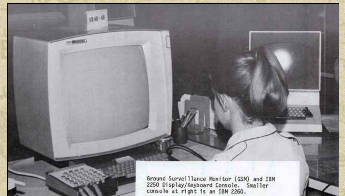
An enemy target (detected by sensor activation) is confirmed through the Ground Surveillance Computer System. (Air Force Historical Research Agency)
