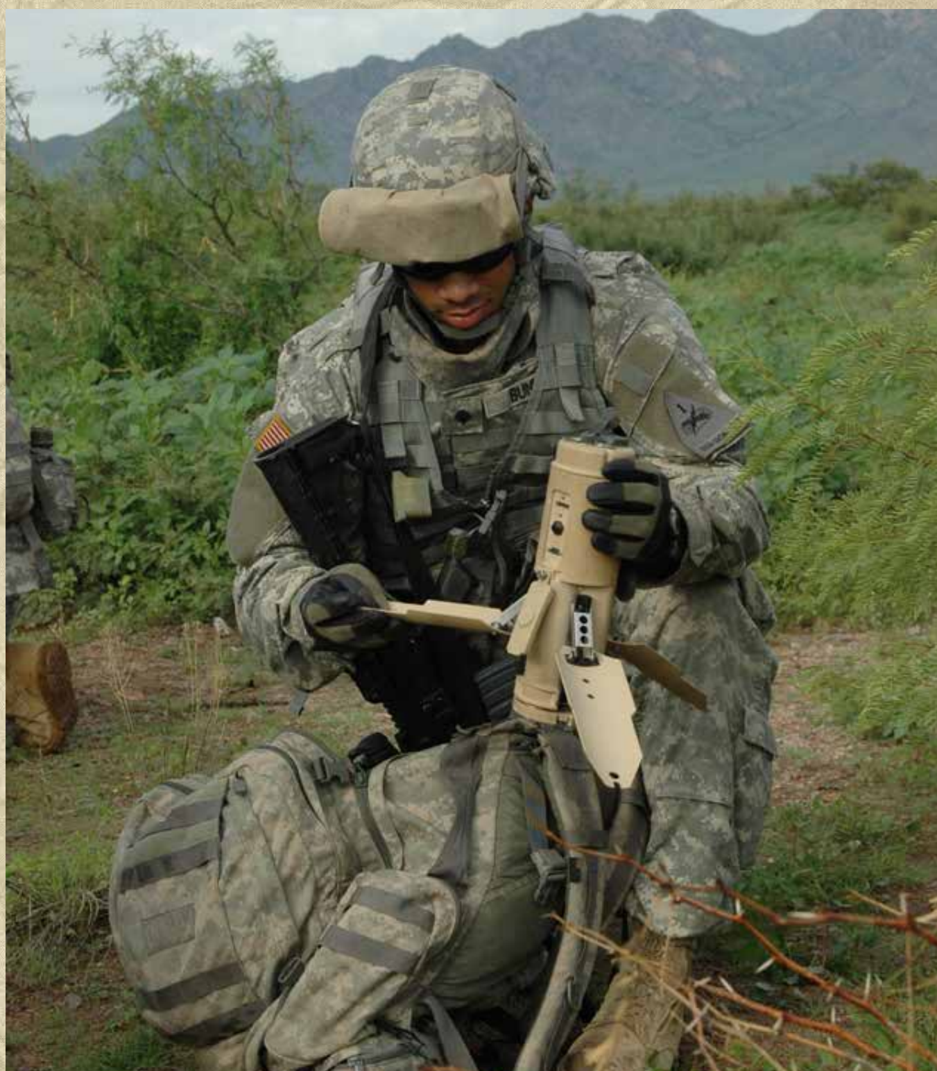
A soldier sets up a tactical unattended ground sensor to monitor an area his unit just cleared. Through seismic, acoustic, radiological, and electro-optic nodes, enemy personnel and vehicles are detected, tracked, and identified. (U.S. Army)
